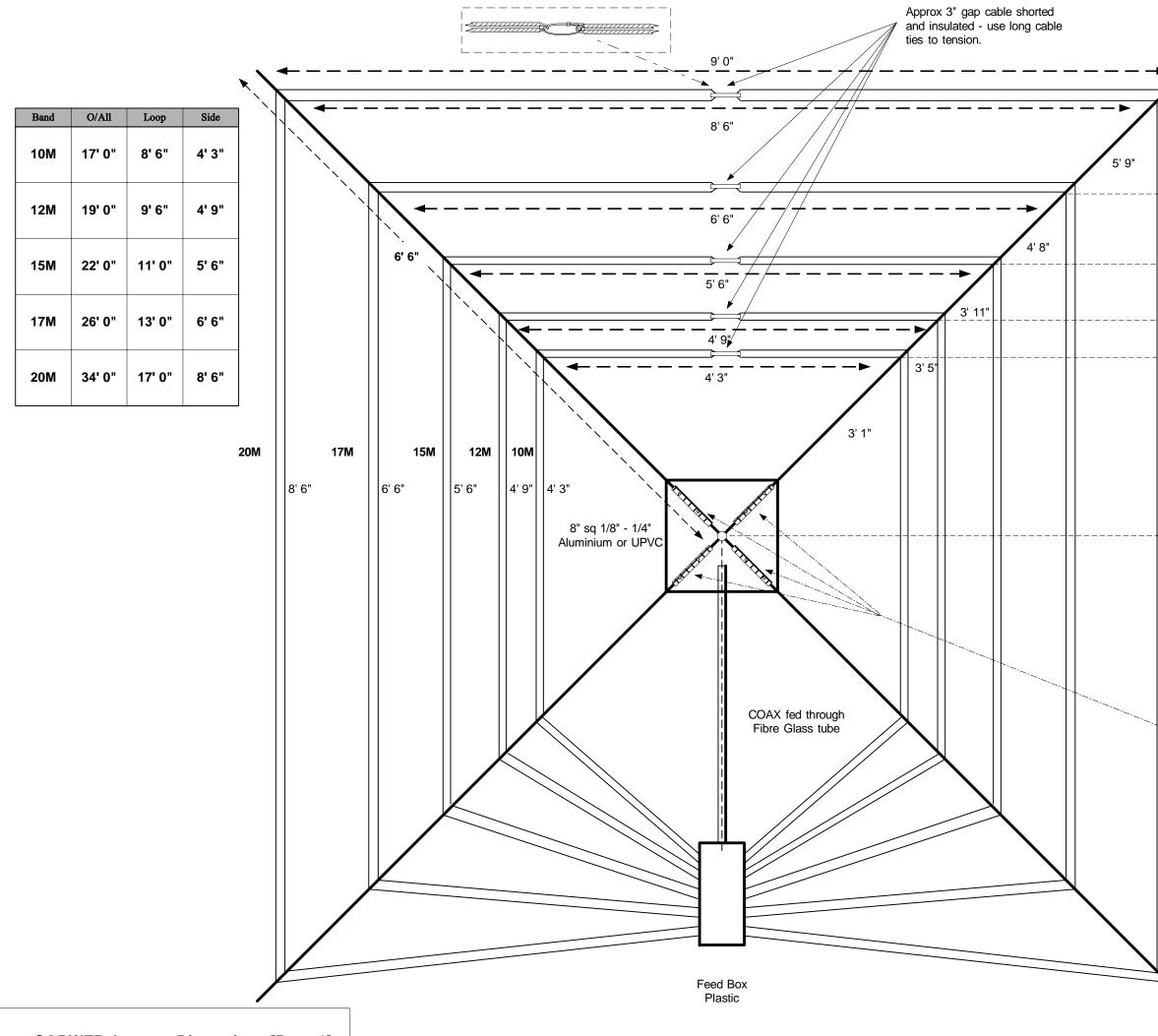
5' 9" 4' 8" 3' 11" 3' 5" 3' 1" Aluminium tube split down the centre for approx 6" to mount the spreaders to the base plate. To strenghten the spreader at the mounting points remember to insert a 6-9" length of wood doweling inside the fibreglass. FibreGlass Base Plate
